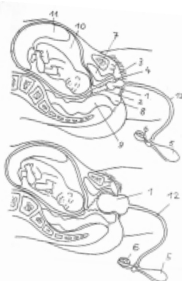
Fig. 2 a: Inserted balloon in a non-dilatated condition. b: Inserted balloon inserted in inflated condition 1= balloon, 2= vagina, 3= vulva, 4= hymen border area, 5= hand pump, 6= manometer, 7= bladder, 8= M. sphincter ani, 9= rectum, 10= amnion, 11= placenta, 12= connecting tube (derived from the patent application for Epi-No®)
